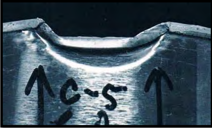
Photo 5: Severe double seam dent plate fracture.
