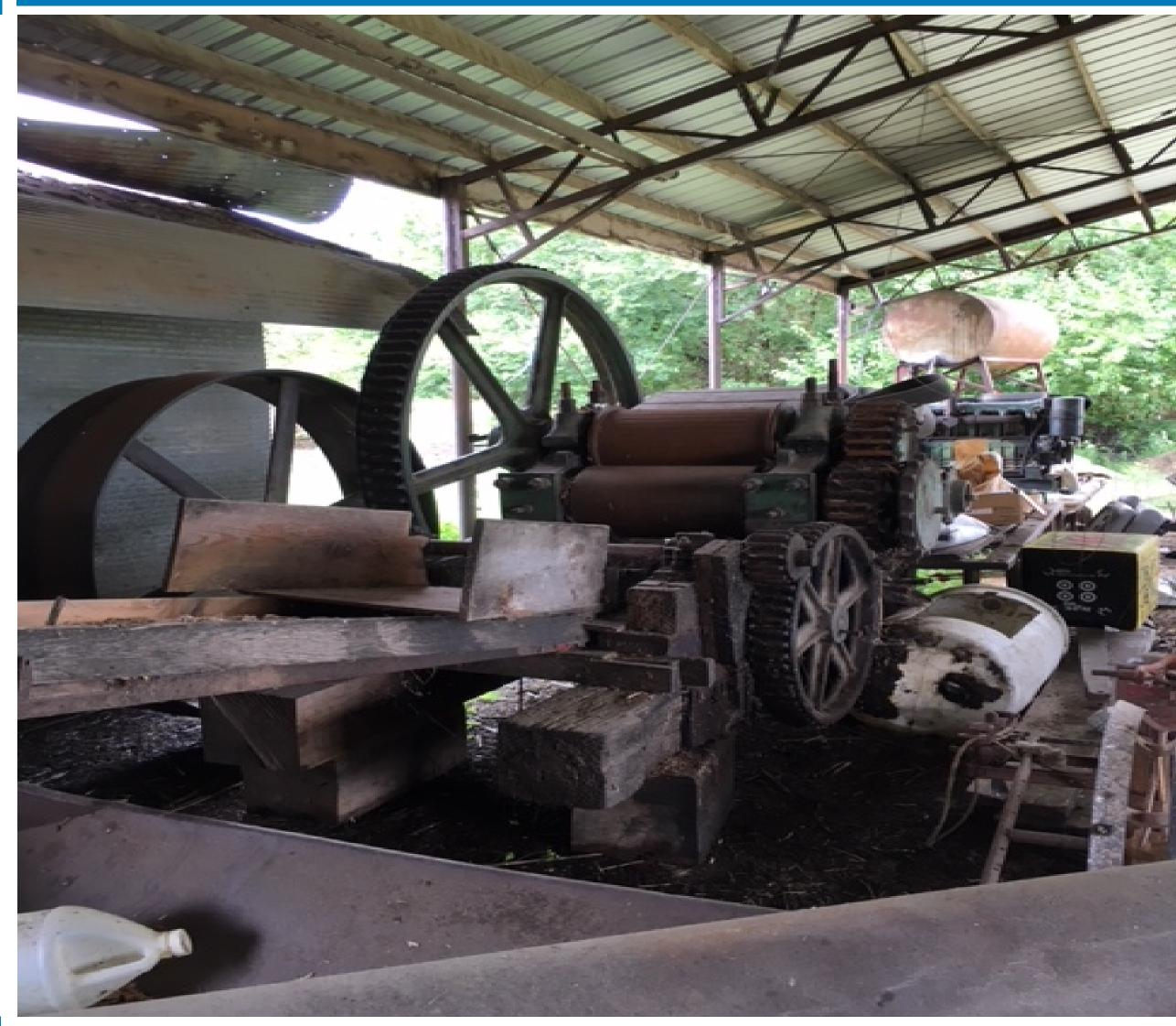
This photo shows machinery on a farm processing facility where sorghum from the fields is squeezed.
