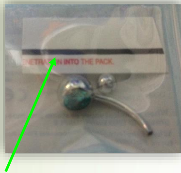
Indicator strip inside sterilization package
