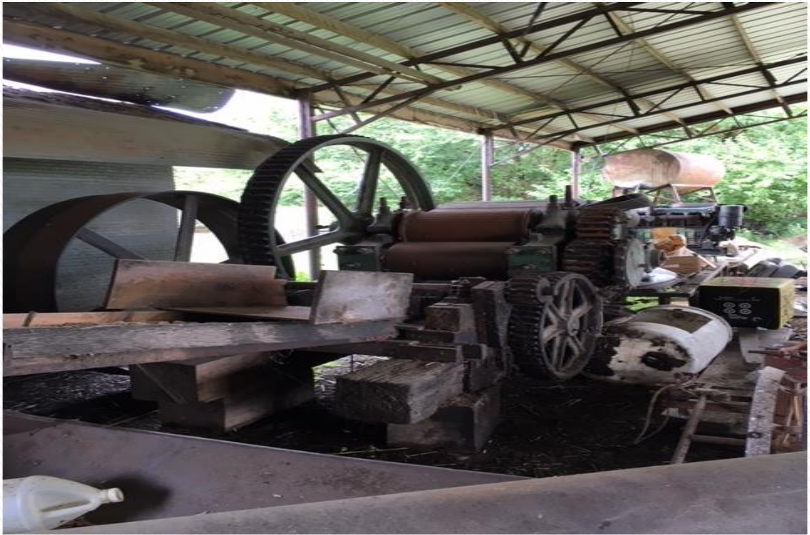
This is the Machinery Used to Squeeze Juice from the Sorghum Plants
