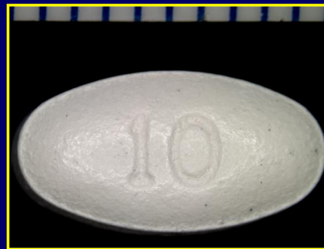
Suspect w/ poor debossing & thicker bevel
