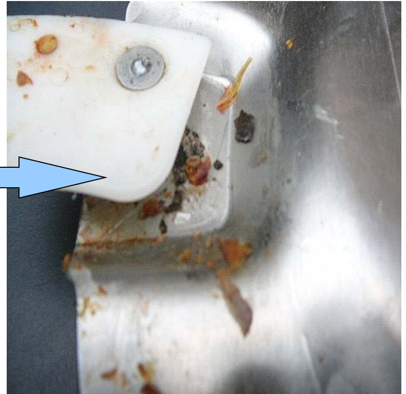
Non-removable, non-cleanable white plastic on inside of blade guard was Salmonella + PFGE match to outbreak
